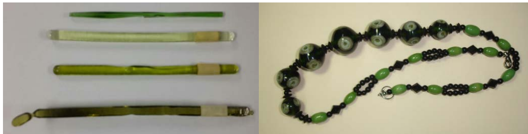
Figure 8: (Left) emerald green glass rods from Krabi sand and (right) beaded necklace made from the emerald green glass rods.
