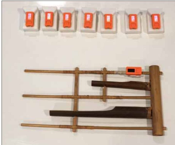
Figure 6. Smart Band devices: showing both the sensor attached to the angklung and the hand-glove vibrator units above.
