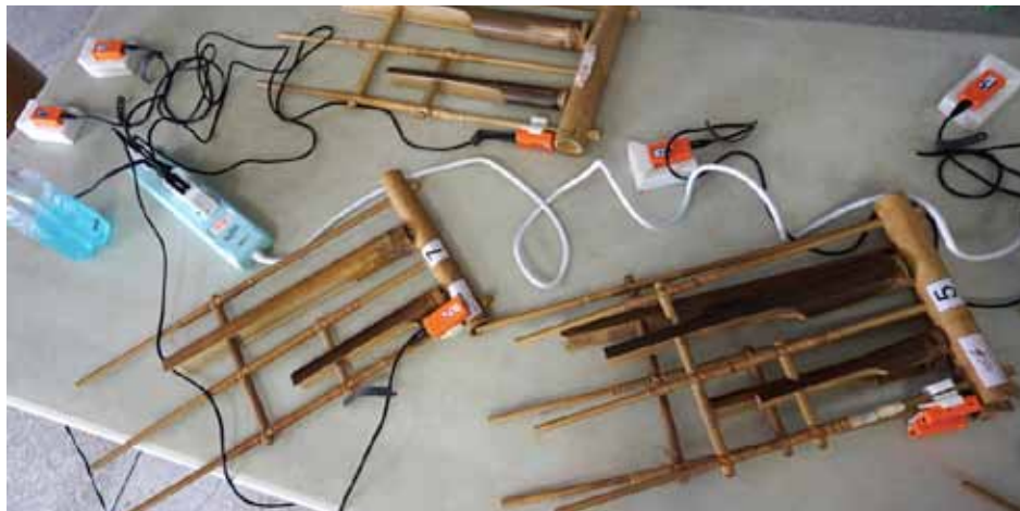
Figure 7. Shows the Smart Band devices being attached to the instrument via wired connections.
