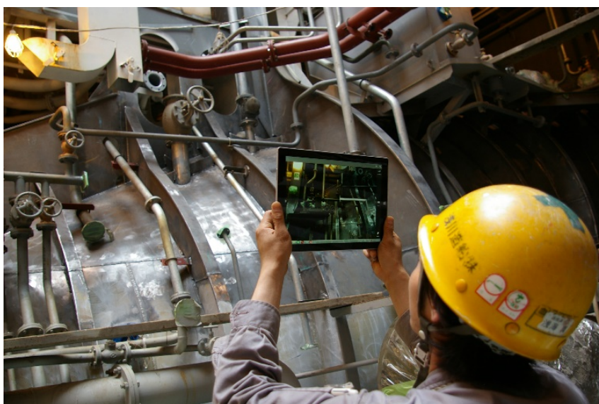
Figure 18 Augmented Reality in ship construction Source: NMRI.
