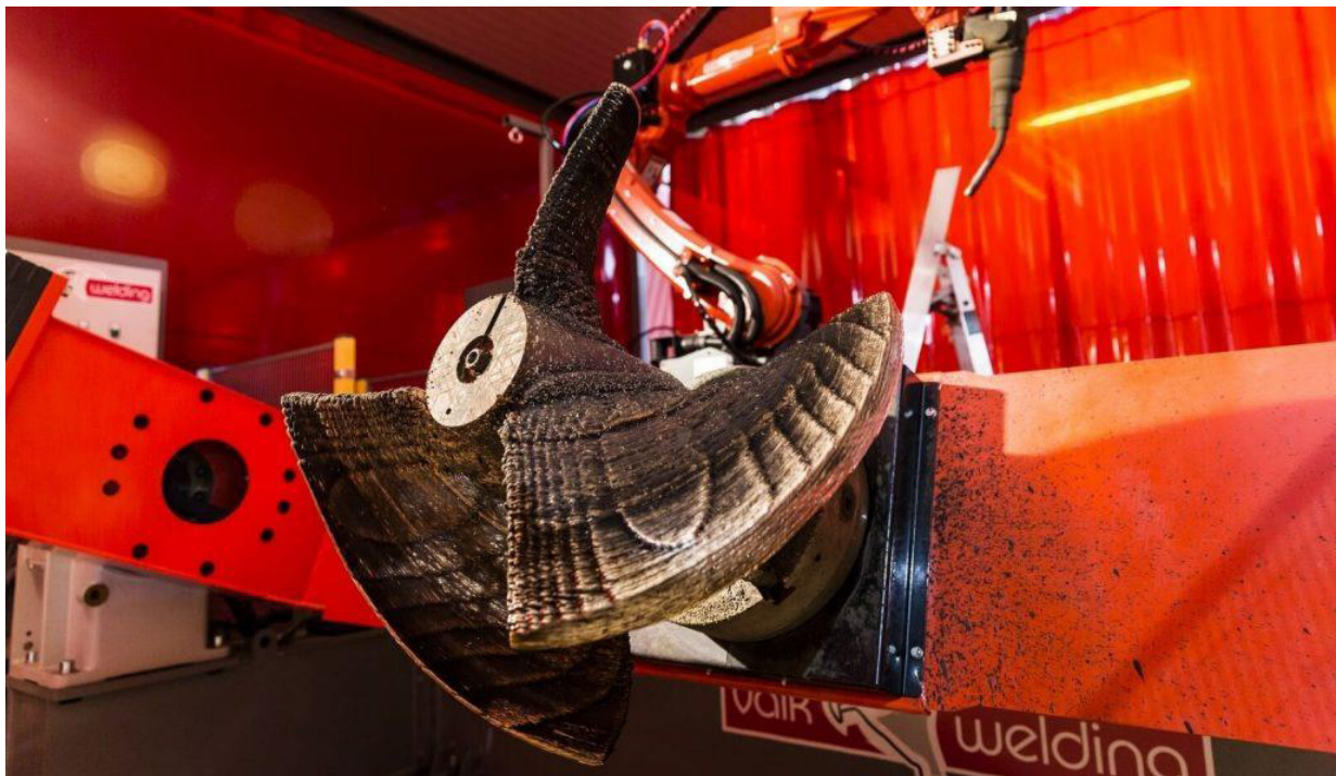
Figure 8 3D printed metal propeller, https://3dprintingindustry.com/news/damen-shipyards-worlds-first-3d-printed-propeller-121112 .
