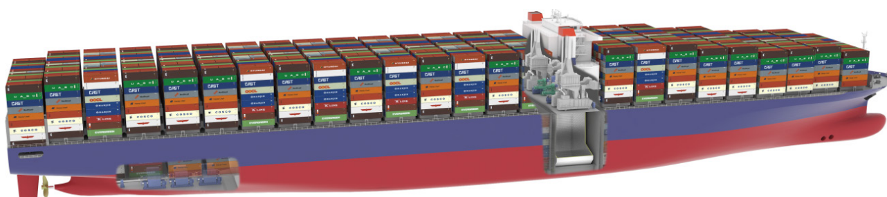
Figure 4 LNG-powered 20,000 TEU containership study PERFECT. Source: DNV GL.
