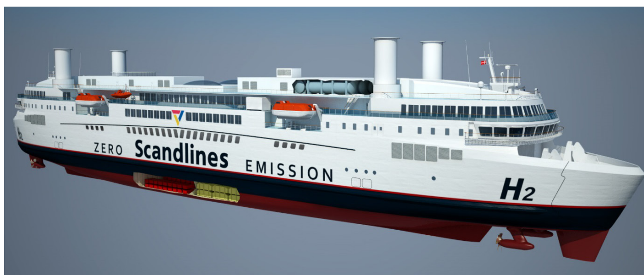
Figure 11 Zero-emission ferry design with fuel cells and batteries, supplemented by Flettner rotors harnessing wind energy; Rohde et al. (2013).
