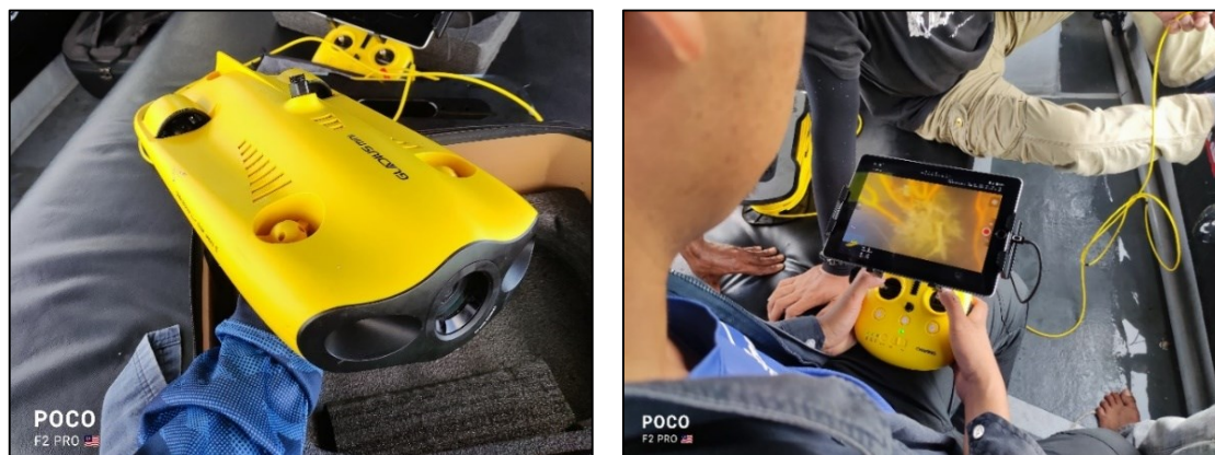
Figure 14 The Gladius Mini ROV is used by the surveyor to obtain visual images of potential locations.
