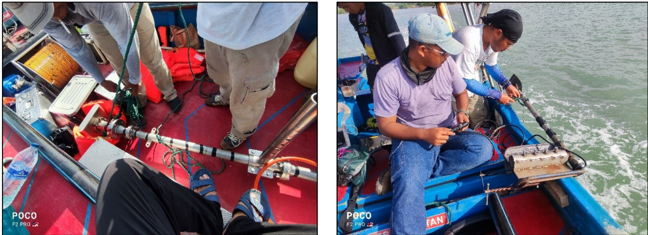
Figure 9 Preparation of INNOMAR 2000 Sub-Bottom Profiling survey equipment- SBP (Pinger system) is placed to the side of the boat before the study is started.
