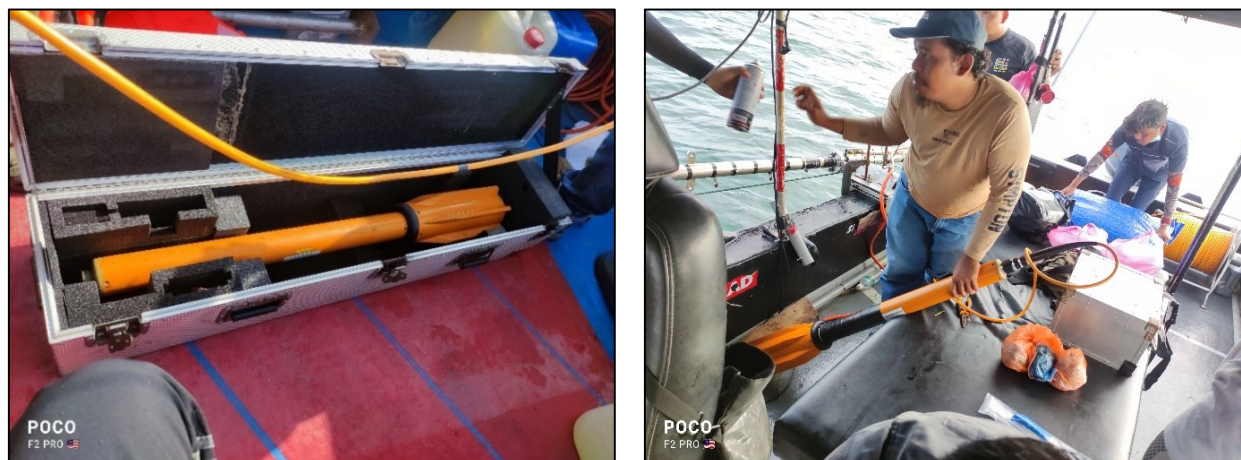
Figure 11 Preparation of SEA SPY 2 Magnetometer device to be towed at the back of the boat before the study begins.
