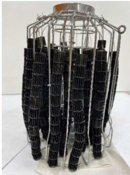
Figure 6 Biofilm carriers in cylindrical form.
