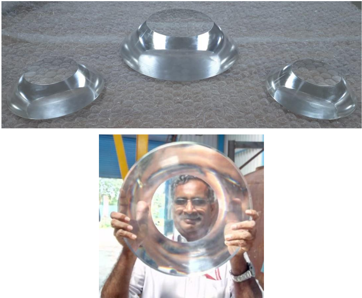
Figure 4 Photos of primary and secondary viewports manufactured and readability inspection by Dr. G. A. Ramadass.
