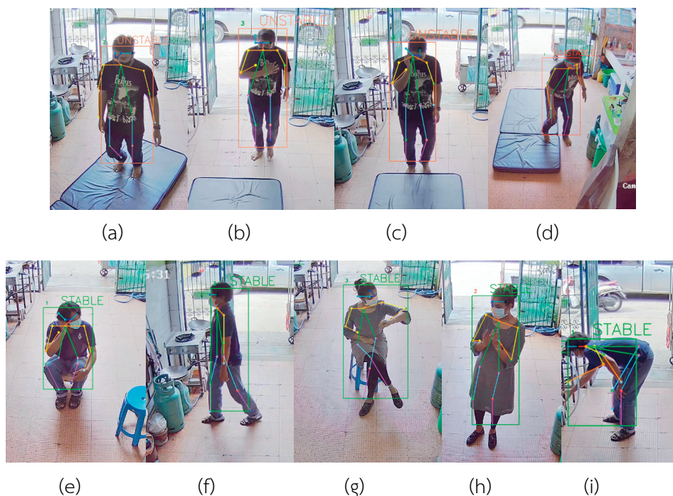
Figure 10 Sample correct stable/unstable motion classification results. (a - d) Unstable motion classification. (e - i) Stable motion classification.
