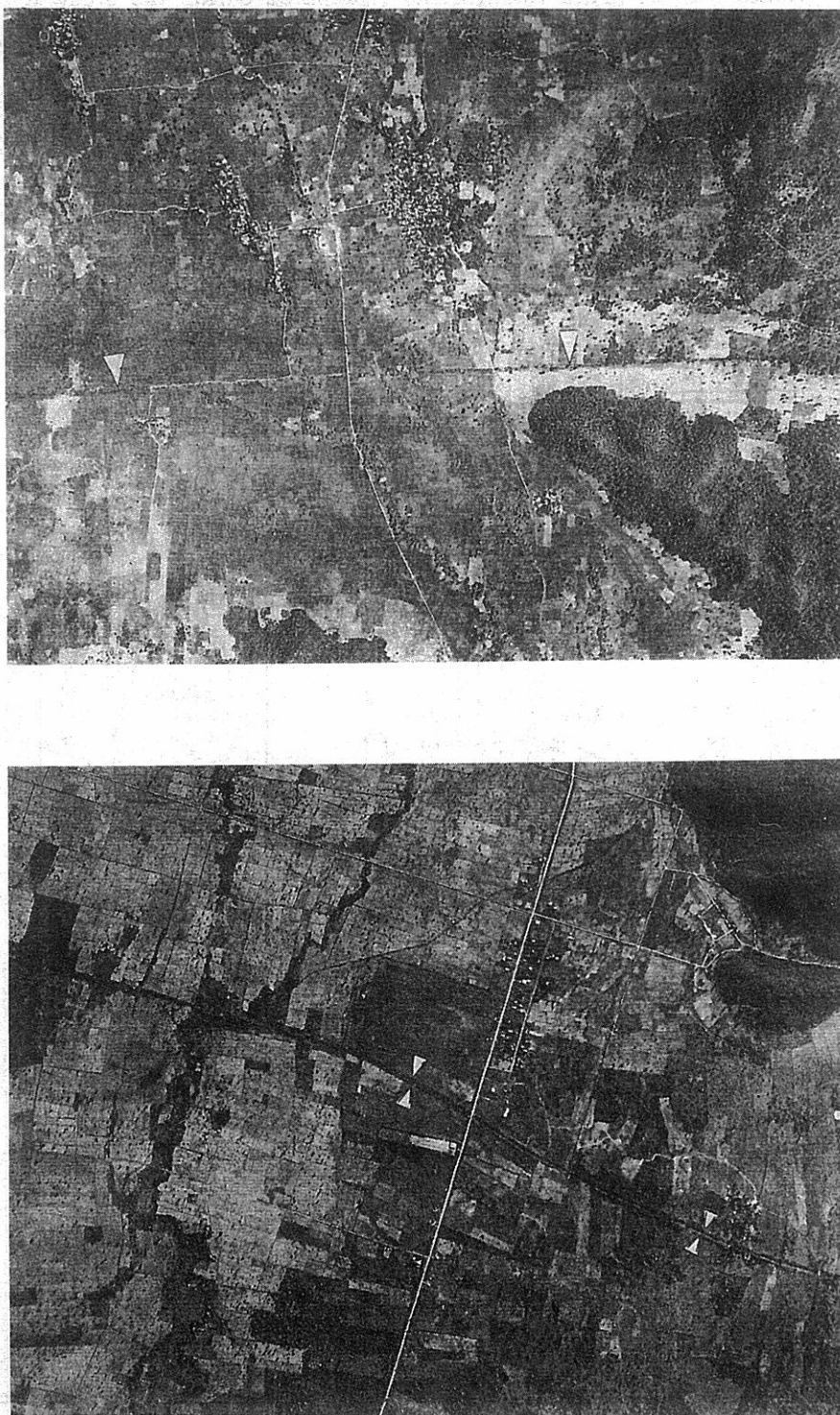
Figure 3. Aerial photograph demonstrating a canal with double embankments (left), and a canal with single embankment (right).
