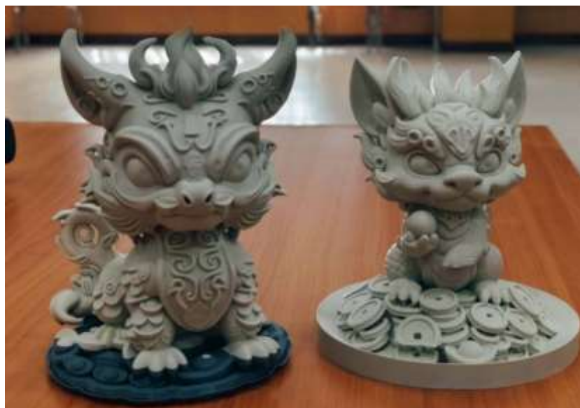
Figure 6: 3D printed characters in PLA+ filament. The physical prototype produced from the finalized 3D model, used as the basis for the Phase 3 expert evaluation reported in Section 3.3.
