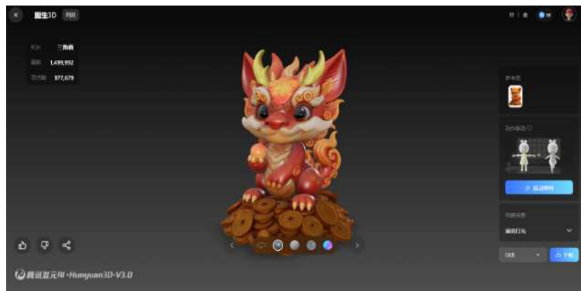
Figure 3: 2D image imported to the Hunyuan AI 3D modelling app to create a 3D model. This step converts the flat character design into an initial 3D mesh, preserving key morphological features such as the dragon-scaled body and single horn for further refinement.
