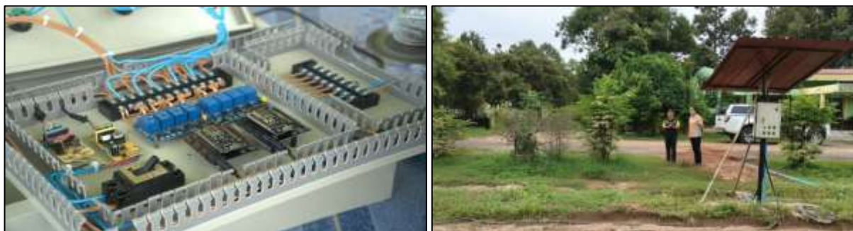
Figure 8: device control box for the smartdrip irrigation system for large-fruited bird's eye chili production to enhance the potential of farming communities engaged in large-scale chili cultivation.
